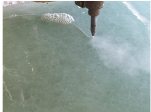
glass panel is sufficient. In both cases the supporting base layer prevents the abrasive corundum from damaging the base of the glass. This is essential for panels, which are to be polished from both sides. The feed rate is determined according to the required edge shape. A feed rate of 150 mm/m is sufficient for roughly sawn edges. Polished or bevelled edges should be cut at a feed rate of 110 mm/m.
